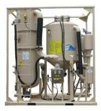
**HOW THEY WORK-** Designed for contained open or vacuum blasting, the VB1200 system blast abrasive through two blasting outlets onto the surface being finished. Our high powered vacuum units, recover the spent abrasive where the dust and waste are separated. The used abrasive is recycled and returned to the storage hopper for re-use.
